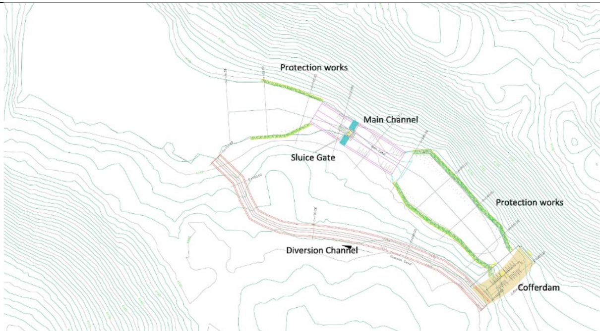
Figure 6. Schematic design of Thulagi Glacial Lake, adapted after full illustration in Annex 26: Technical Lake Lowering Design report.
