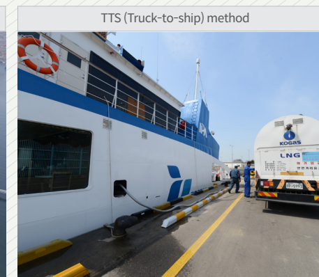
• Using tank lorries, for small-scale supply to LNG propulsion ships at ports
