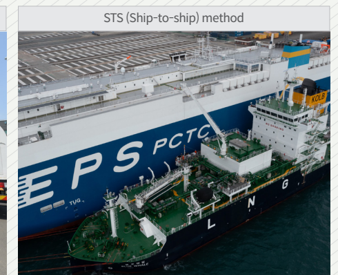
• Using LNG bunkering ships, for medium-scale supply to ships, regardless of vessel type or location
