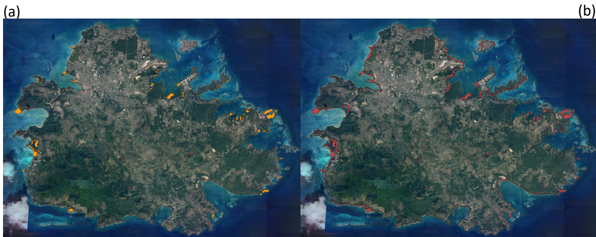
Figure 3: Antigua’s coastline changes under 0.13 m Sea Level Rise (SLR) scenario (a), and 1.45 m Sea Level Rise (SLR) scenario (b)
